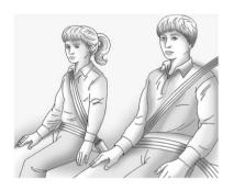
Older children who have outgrown booster seats should wear the vehicle safety belts. The manufacturer's instructions that come with the booster seat state the weight and height limitations for that booster. Use a booster seat with a lap-shoulder belt until the child passes the fit test below:
